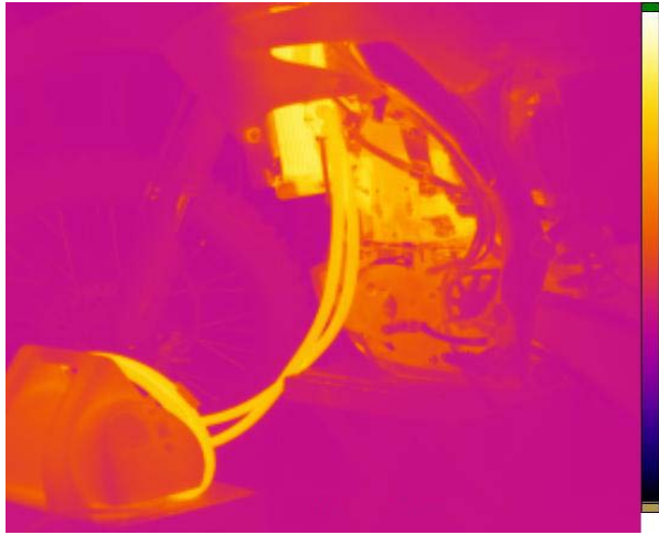
Figure 1 A thermal image of a preheater heating a single-cylinder engine. The vertical bar at right indicates the temperature gradient.
