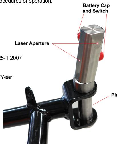
Remove the kingpins, spindles and adjustors from the yoke. Insert the Sniper pins into the yokes and fit the head unit onto the pins.
